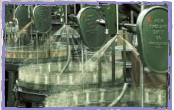
Our extensive braiding lines feature braiders with 8, 12, 16, 24 and 48 carriers.
